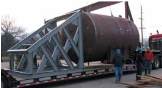
UN PORTABLE VESSEL FOR TRANSPORTING CHEMICALS
